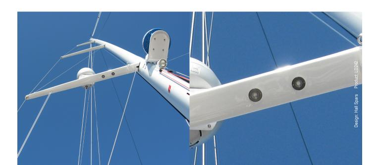
This has been specifically designed for use on yacht spreaders to illuminate the deck or other spreaders below. It is fitted with the latest LED technology and machined from a solid billet of high grade aluminium. This is hard anodised making it resistant to harsh sea environments. The narrow 12 degree beam will light a deck from 9m.
